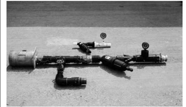
**Screen filters, pressure regulators, and pressure gauges**
